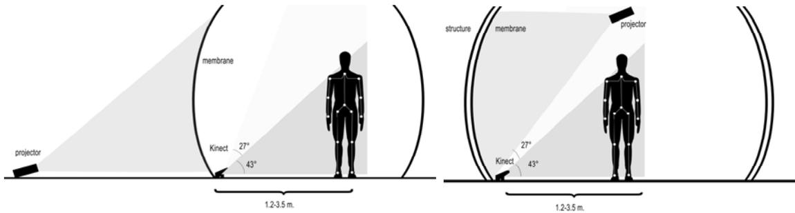
**Figure 4. Two alternative setups of portable immersive environments that combine textile structures, projections and the Kinect sensor.**
