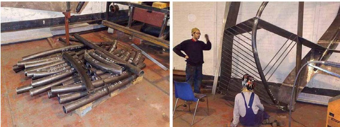
Fig. 9: Pipe Segmentation
