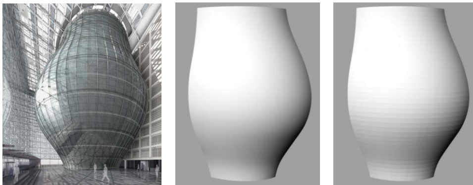
Figure 12a, b and c: The initial design, a quarter of the surface geometry and the section described by single curved panels. (3a Computer rendering polygon graphics 2008 by Philippe Samyn and Partners architects & engineers, Lead and Design Partners)
