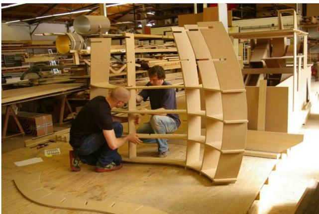
Figure 5. Shelves, Design and Engineering: Ivo Vrouwe. An example of Phase 1; Volume patterning reframed into a surface-active system by the use of wood.
