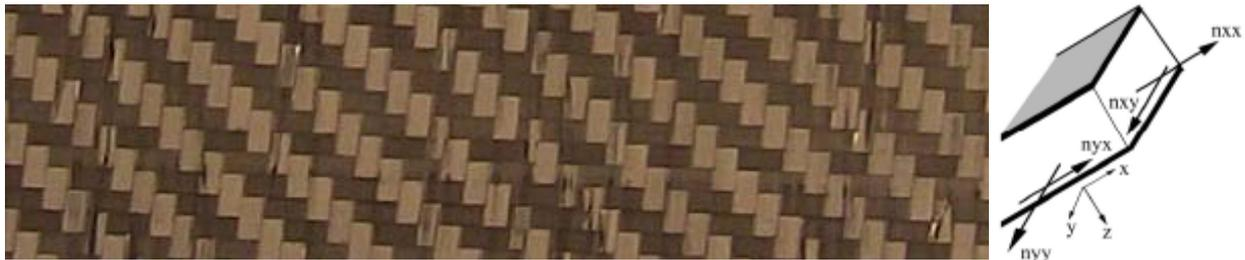
Figure 3: Woven PP sheet, internal membrane forces
