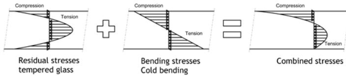
Figure 2: Superposing pretensions stresses and bending stresses
