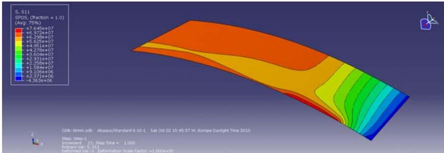
Figure 6: Typical bending stress (stresses in tangential direction) of a cold bent panel in end situation.
